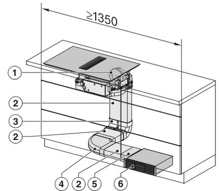
KMDA7676-1FL, KMDA7876-1FL, KMDA7676FL, KMDA7876FL – Einbauvariante 4 Umluft
