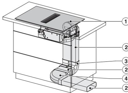
KMDA7676-1FL, KMDA7876-1FL, KMDA7676FL, KMDA7876FL – Einbauvariante 3 Basis – Skizze
